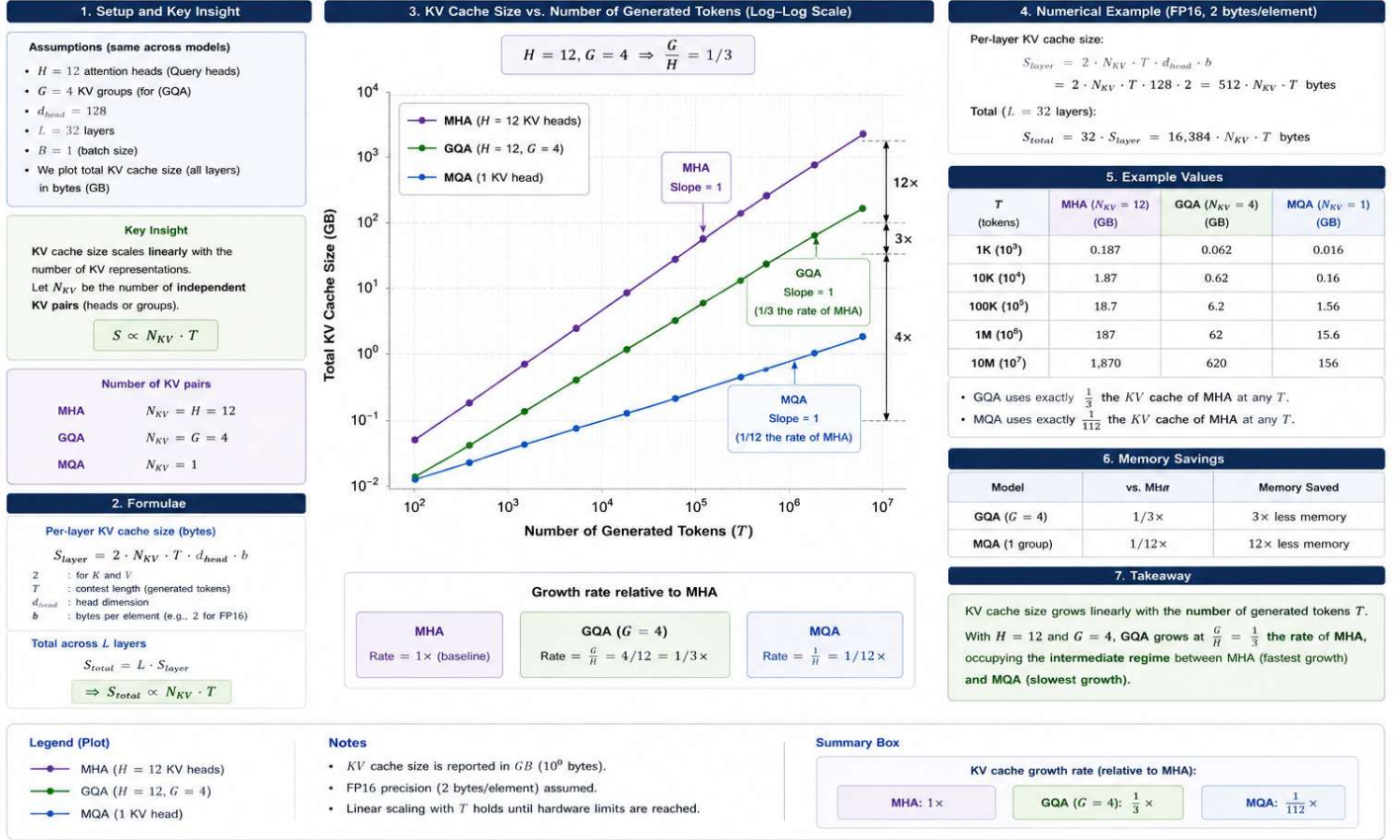
Figure 12 — KV cache growth under MHA, MQA, and GQA ( H = 12, G = 4 ) as a function of generated tokens: GQA occupies the intermediate regime between MHA and MQA, growing at \frac{G}{H} = \frac{1}{3} the rate of MHA
